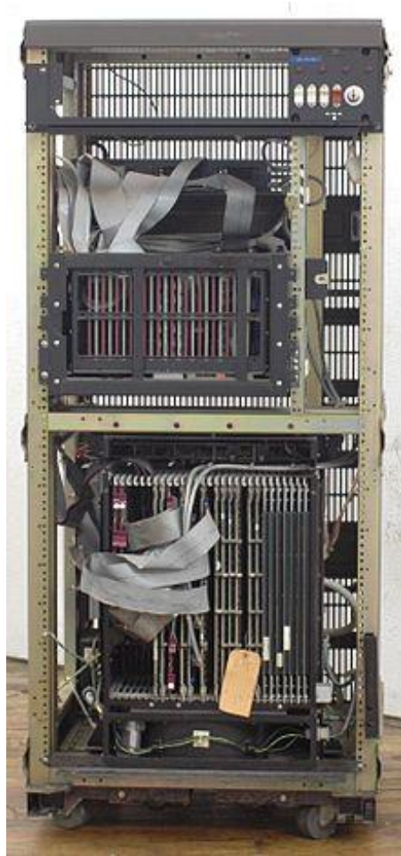
Figure 2 – DEC KS10 with Covers Removed (photos from RCIM)
