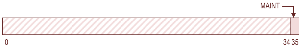
Figure 50 – IO Bridge Maintenance Register (UBAMR)
