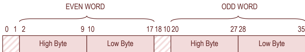
Figure 45 – IO Bus Byte and Word Translation
