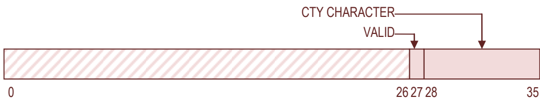
Figure 40 – KS10 CTY Output Word (KS10 Memory Address 000033)
