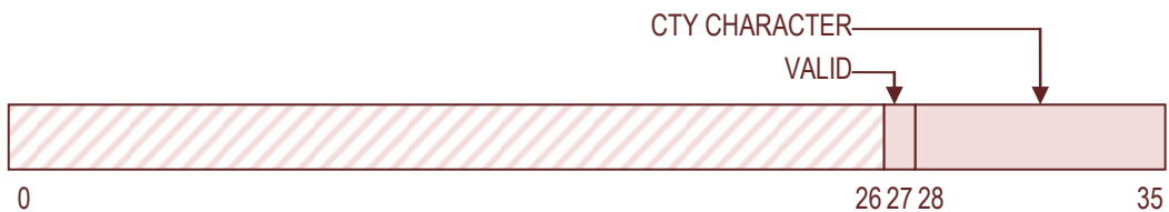
Figure 39 – KS10 CTY Input Word (KS10 Memory Address 000032)
